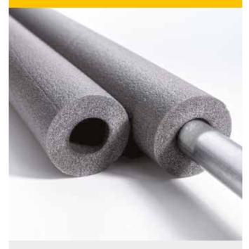
Polyethylene Insulation is an economically priced insulant with self extinguishing fire characteristics, which is used for many plumbing and domestic installations. The key benefits of this type of insulant include a closed cell structure, low weight, a clean finish, ease of installation, flexibility, resilience, and a relatively low cost.
