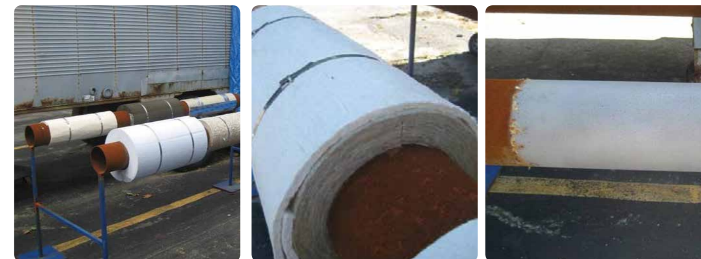
90 day CUI tests with Pyrogel® XT on its own and in conjunction with other products
