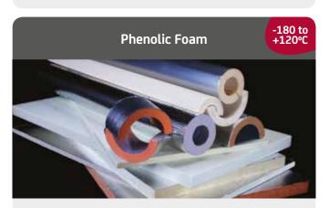
Phenolic Foam is a rigid foam with a strong resistance to burning and the spread of flames. It also has the lowest thermal conductivity of any commonly available rigid foam insulant at 0.025 W/m/°K.
