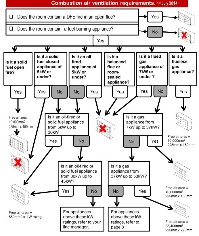
All vent dimensions are nominal sizes only. Free air will vary by manufacturer. Verify that the vent provides the required free air. The free air is often embossed into plastic vents
